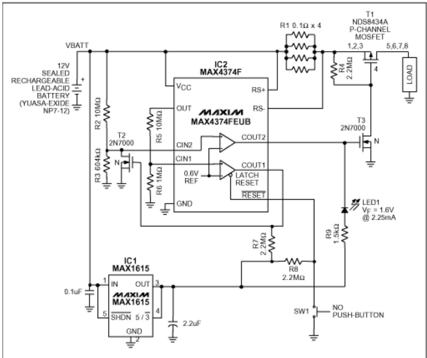
Figure 1. A fault condition (battery terminal voltage <10.5V or battery current >5A) causes T1 to open and LED1 to illuminate.
