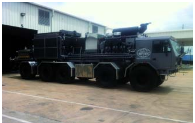
Figure 2: The supercapacitor on this oil drilling truck enables it to restart its engine reliably after long periods drilling for oil in remote areas and in spite of extreme temperatures.
