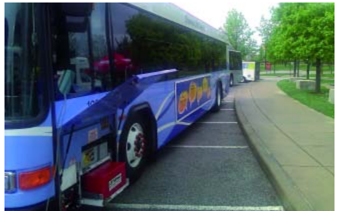
Figure 1: Frequent stop-start operations on bus services do not impact the reliability of buses when a supercapacitor supplies engine starting power
