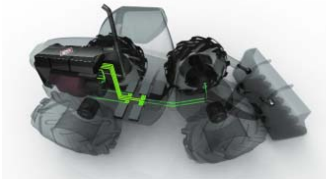
Figure 1: Electrified wheel-loader: serial configuration permits 20,000 litres of fuel to be saved annually at 4000 operating hours.
