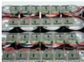
Figure 4: Internal construction of the WIMA SuperCap module with actively balanced single cells.
