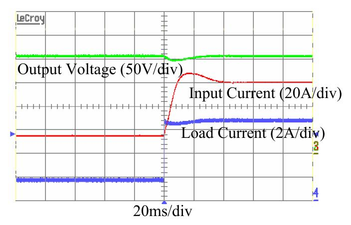
With voltage control loop bandwidth designed at 20 Hz, settling time is about 40ms under load step
