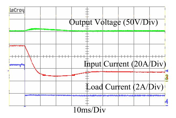
With voltage control loop bandwidth design at 20 Hz, settling time is about 40ms under load dump
