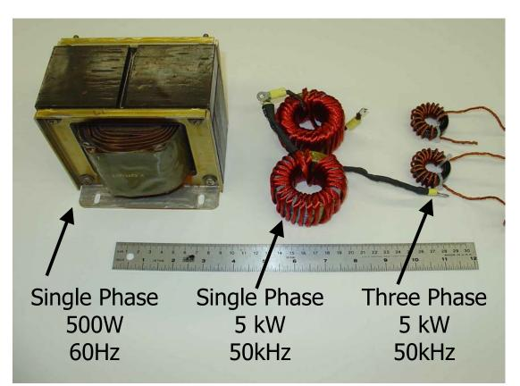
With V6 converter, an effective 10x reduction in DC link filter inductor in terms of cost, size and weight
