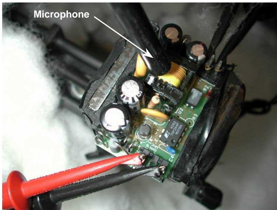
Figure 11. Test Arrangement for Audio Noise Measurement
