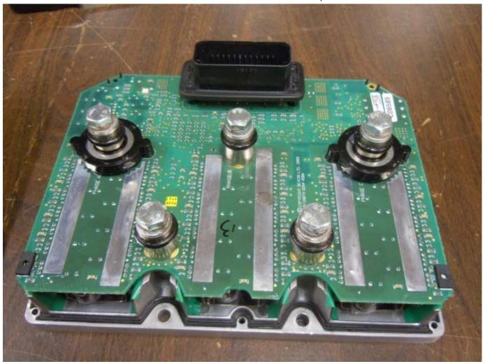
The FETs are clamped to the heatsink by spring clamps. These must be held open with a special jig during assembly while the top board is inserted.
