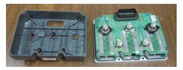
Just one big board. Surprisingly there are no bus bars, the 350A connections go directly to the PCB! The three half bridges are clearly visible. Each leg uses seven IPP075N15N3 G 150V 7.5mOhm FETs.
