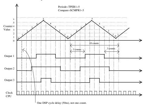
Note: the first period of a continuous up/down count is 1 DSP cycle longer and is not totally symmetrical (see diagram above).
