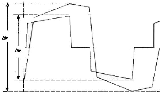
Fig 13. - Primary Current - ZVT vs Square Wave
