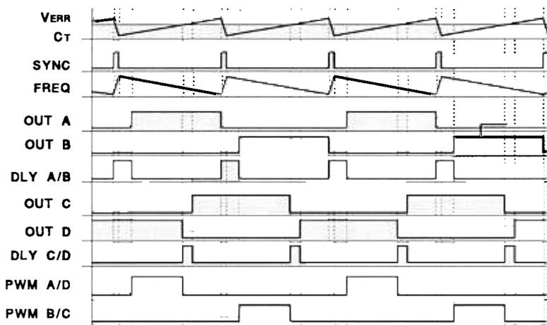
Fig 3. - Phase Shifted PWM Control Waveforms
