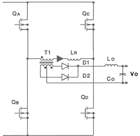
Fig 1. - Full Bridge Topology - General Circuit
