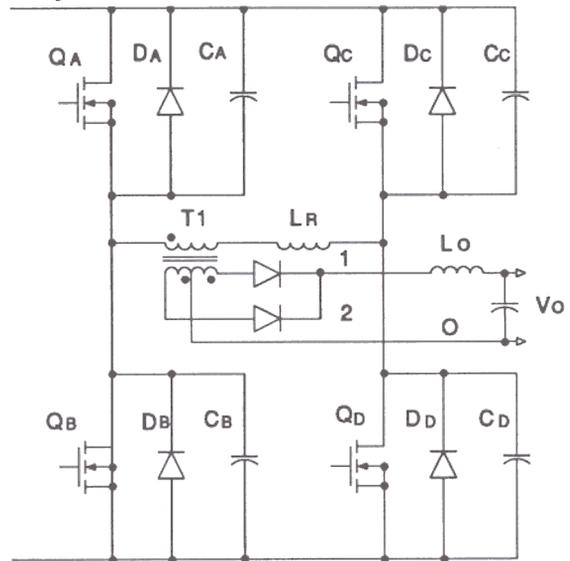
Fig 5. - Phase Shifted PWM Switch Orientation
