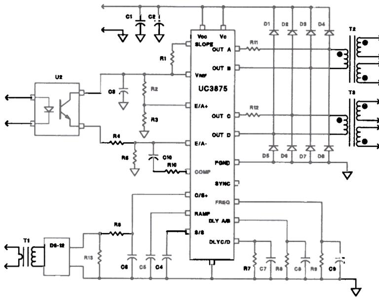
Fig 15. - Control Circuit Schematic
