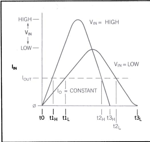
Fig. A6 -  $i_{in}$ ,  $t_{on}$  vs. Line Variation
