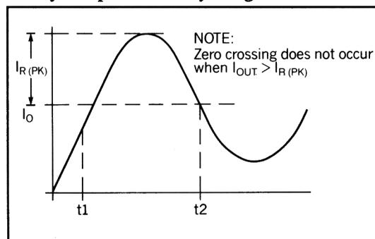
Fig. 9 - Input Current - No Zero Crossing
