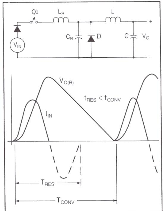
Fig. 12 & 13 - Resonant Mode Buck Regulator
