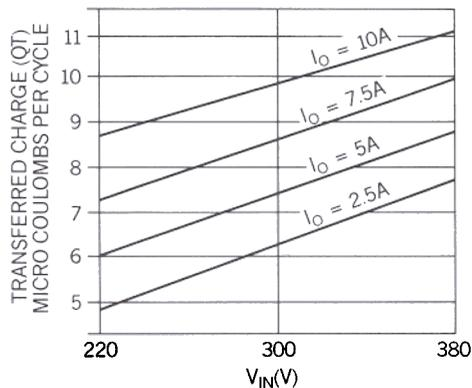
Fig. 19 -  $Q_b$ , Transferred Charge vs.  $V_{in}$  and  $I_{out}$
