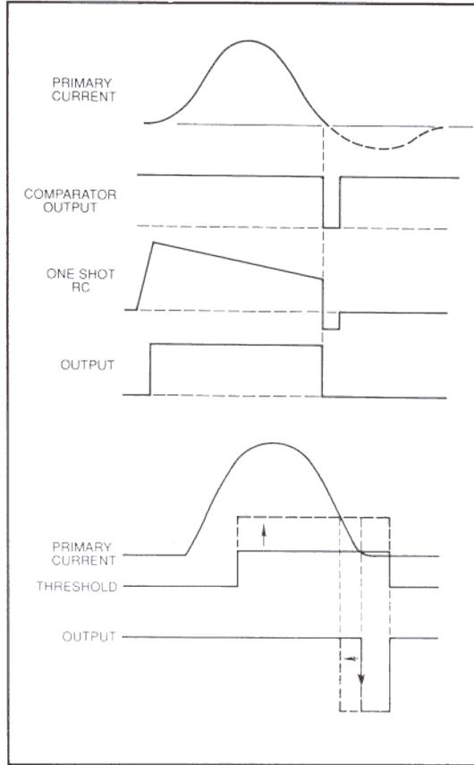
Fig. 24 & 25 - Zero Current Switching
