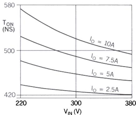
Fig. 18 - On Time vs.  $V_{in}$  and  $I_{out}$
