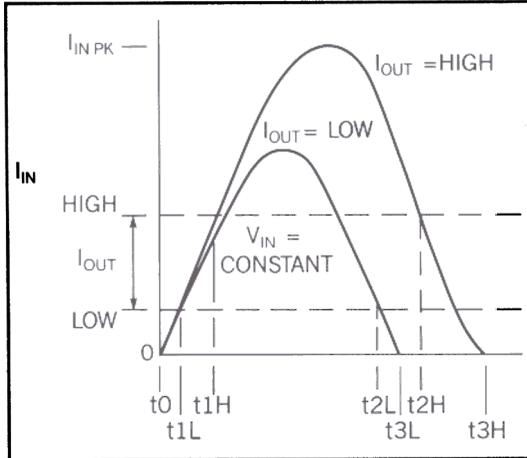
Fig. A7 -  $i_{in}$ ,  $t_{on}$  vs. Load Variation
