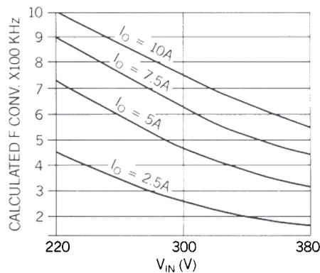
Fig. 21 - Calc. Conversion Freq vs.  $V_{in}$  and  $I_{out}$
