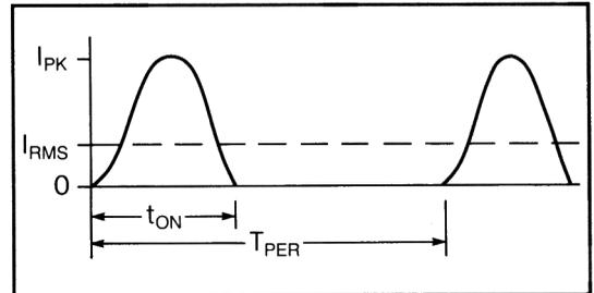
Fig. 17 - rms Current Calculation
