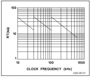
Figure 2. Timing Resistor (RT) vs. Oscillator Frequency
