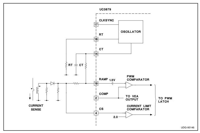
Figure 6. UC3879 with Peak Current Mode Control
