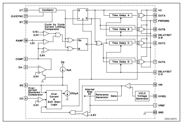
Figure 1. UC3879 Block Diagram
