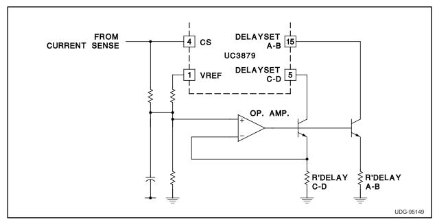
Figure 9. Adaptive Control of Delay Times
