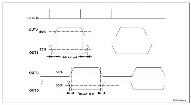
Figure 8. Output Timing Diagram for Steady State Operation
