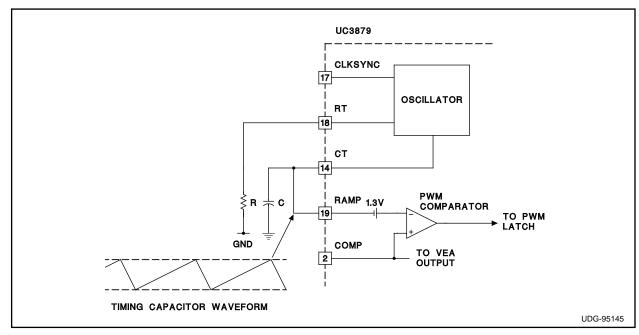
Figure 5. UC3879 with Voltage Mode Control
