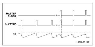
Figure 3. Oscillator Waveforms
