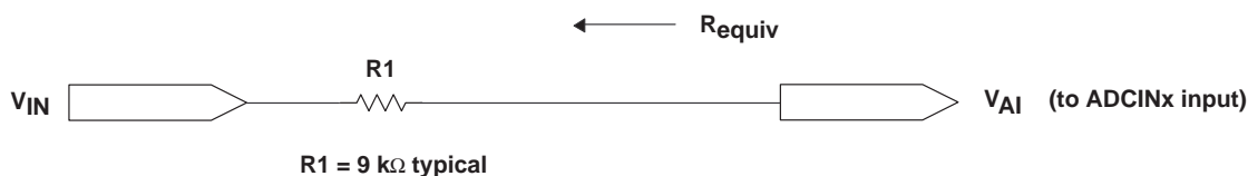
Figure 46. Typical ADC Input Pin Circuit
