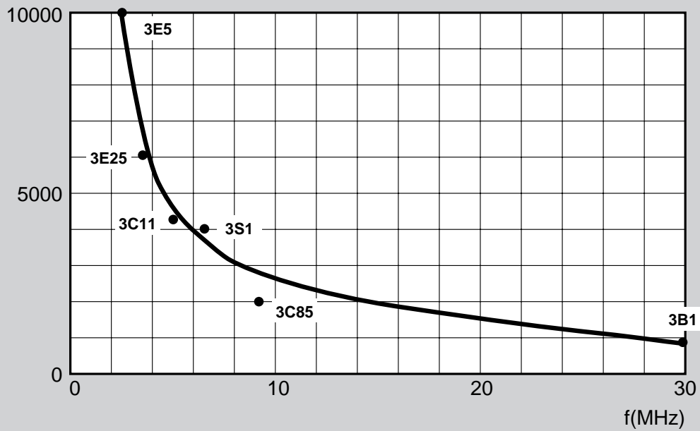
Fig.4 Frequency of impedance peak for some MnZn ferrite materials.
