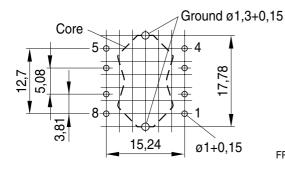
Hole arrangement View in mounting direction
