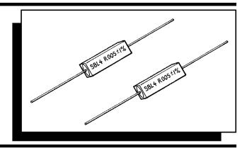
The SBL Series is a low ohmic non-inductive resistor with a low temperature coefficient in a fully insulated ceramic housing. It is ideal for applications in power supply regulation, motor control current monitoring, feedback control loops, overload sensors and radio frequency applications. The solid metal element has welded copper terminals and is encapsulated in a ceramic housing, filled with compressed silica sand.
