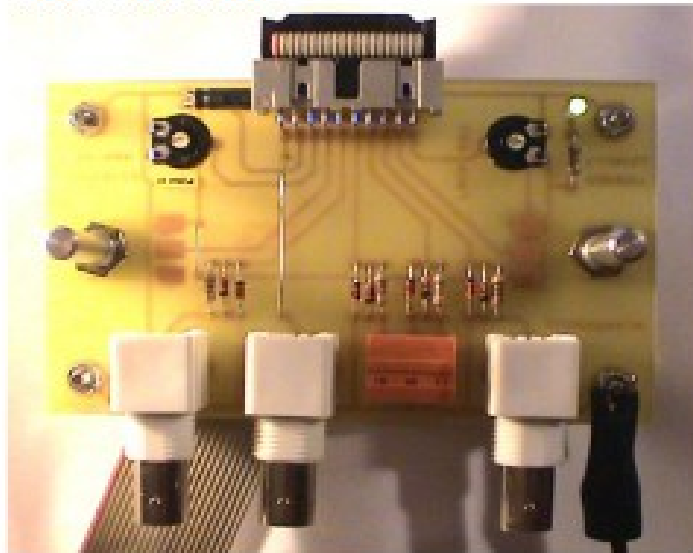
Figure 5.5 Interface analogique de test (images-maquettes [AT8535-ANALOG-12].jpg).
