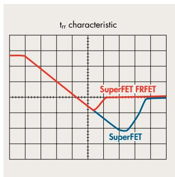
FRFET offers over 50% improvement in diode reverse recovery characteristics ( $Q_{rr}$ ,  $T_{rr}$ ) which is ideal for phase-shifted full bridge topologies (ZVS) and half-bridge/full-bridge topologies (hard switching).
