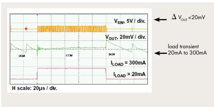
Fast Load Transient DCM-CCM-DCM
