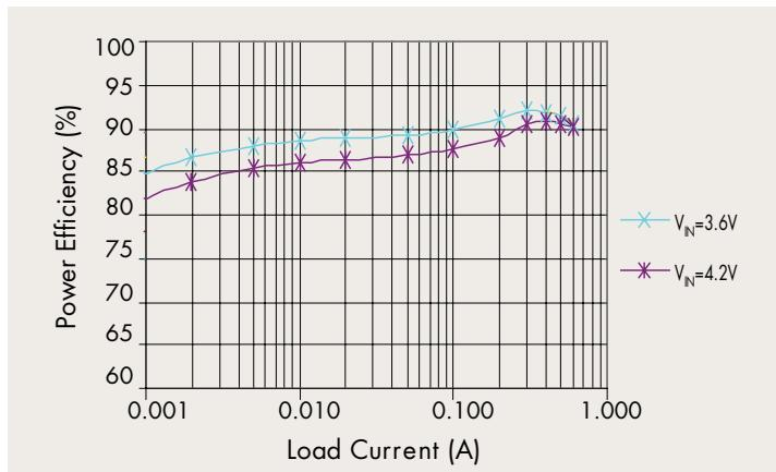
Power Efficiency vs. Load Current
