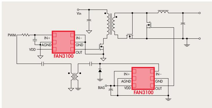
Forward Converter with Hybrid Synchronous Rectifier
