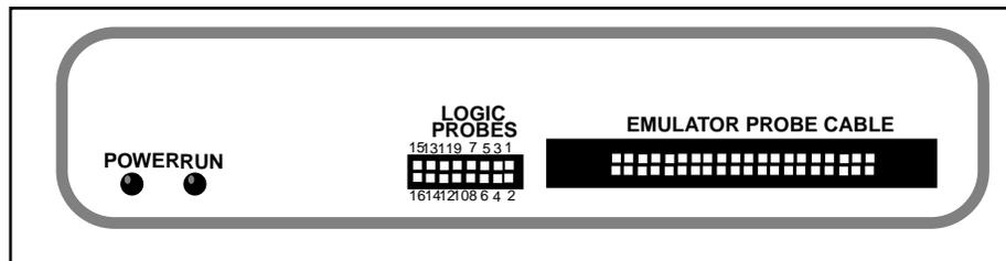
Figure 2.4 PICMASTER Pod Front Panel
