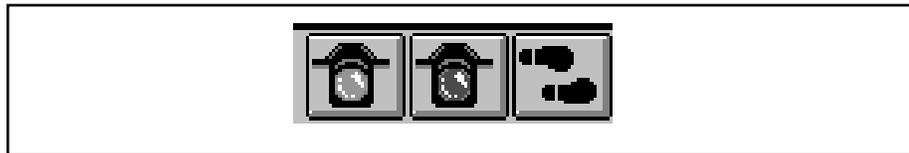
Figure 3.1 Tool Bar Icons: Run, Halt, Step
