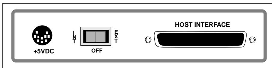
Figure 2.3 PICMASTER CE Pod Rear Panel
