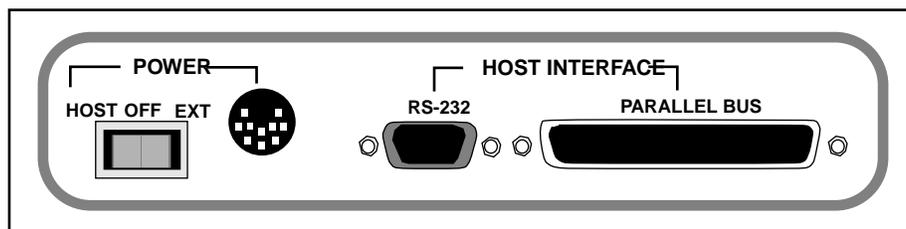
Figure 2.2 PICMASTER Pod Rear Panel
