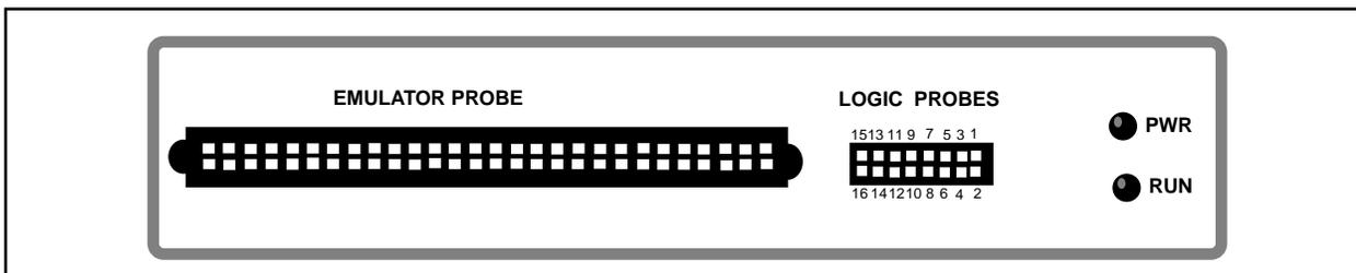
Figure C.3 PICMASTER CE POD FRONT PANEL
