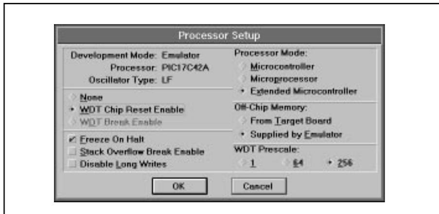
**Figure 4.9 PIC17C4X Processor Setup Dialog**
