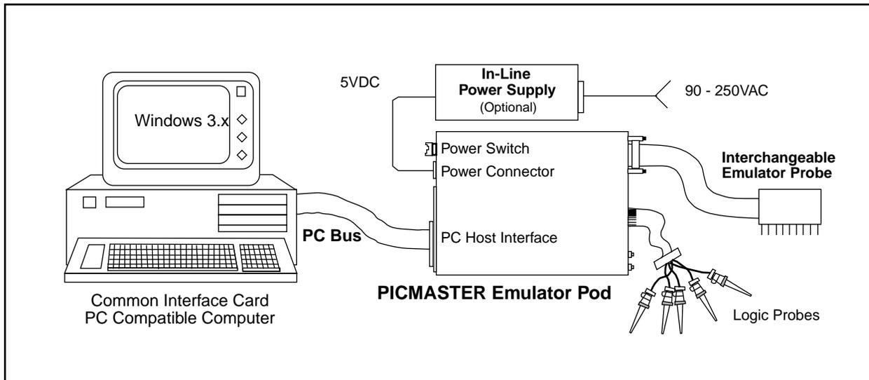
Figure 1.1 Block Diagram of Emulator System
