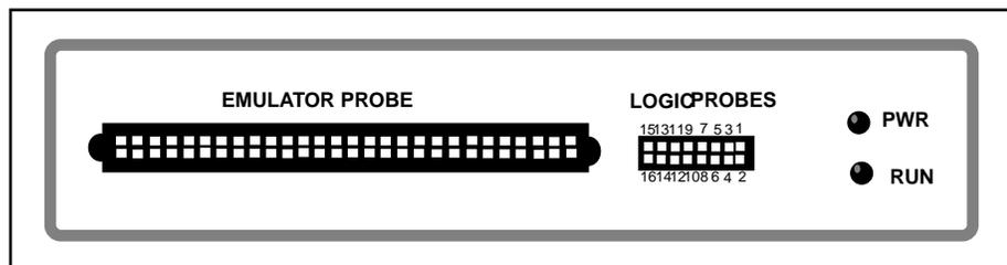
Figure 2.5 PICMASTER CE Pod Front Panel
