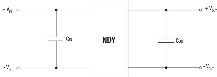
**Recommended circuit for reduced ripple 3.3V output**
