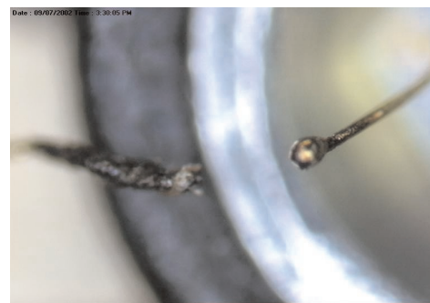
Figure 17. Fused wire failure.
