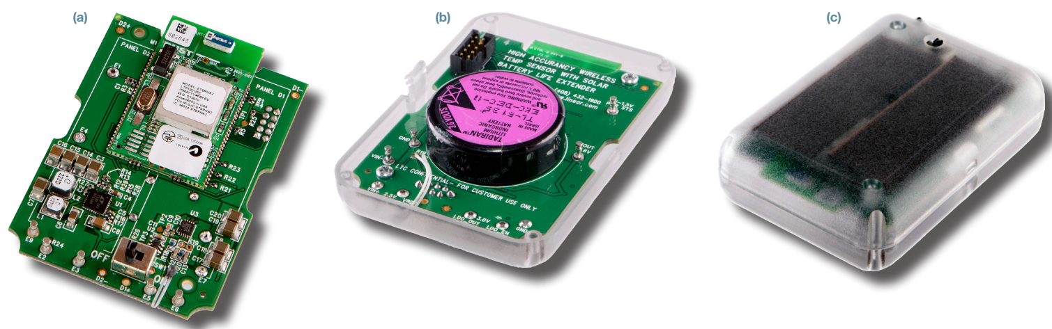
Figure 2. Entire self-contained, self-powered temperature sensor system fits into an enclosure less than seven cubic inches in volume. Battery, solar panel and wireless-networking controller are included. No external wires or connections are required. Installation is easy: place it somewhere. (a) Front of board showing signal chain, power and control circuitry and wireless mesh network module; (b) back of board with battery; (c) complete solution in enclosure with solar panel installed.
