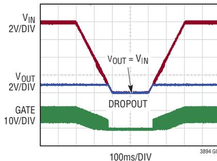
$V_{IN}$  TRANSIENT 12V TO 4V AND BACK TO 12V
