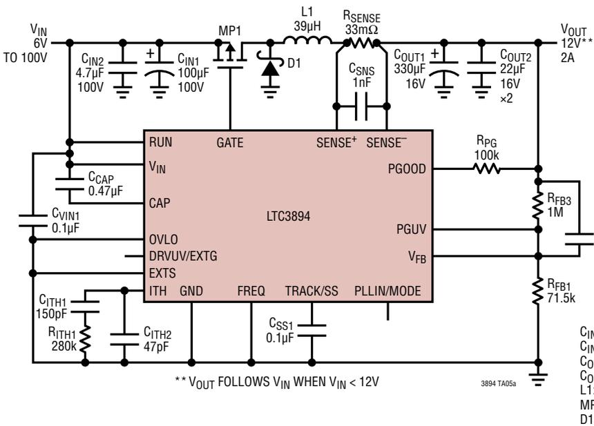
Figure 14. 6V to 100V Input, 12V/2A Output, 350kHz Step-Down Regulator
