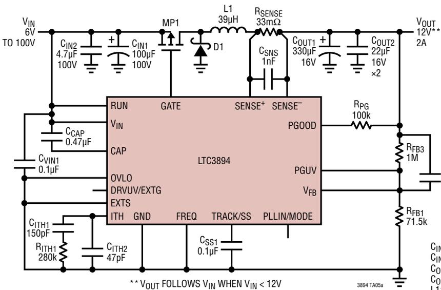
Figure 14. 6V to 100V Input, 12V/2A Output, 350kHz Step-Down Regulator
