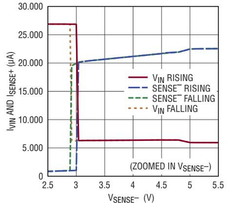
**$I_{VIN}$  and  $I_{SENSE-}$  vs  $V_{SENSE-}$  (Pulse-Skipping Mode)**
