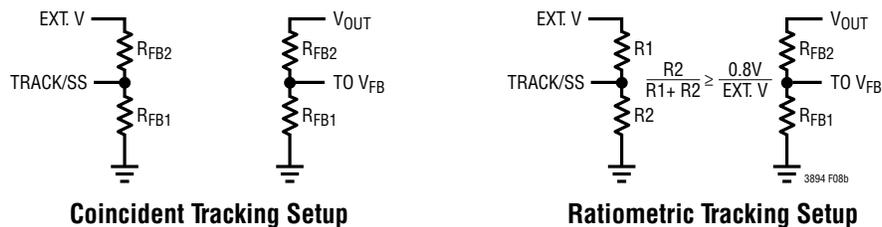
Figure 8(b): Setup for Ratiometric and Coincident Tracking
