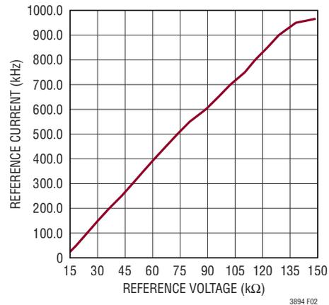
Figure 2. Switching Frequency vs Resistor on FREQ Pin
