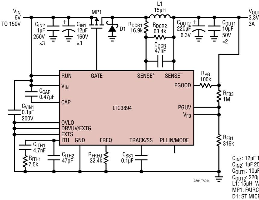
Figure 13. 6V to 150V Input, 3.3V/3A Output, 175kHz Step-Down Regulator
