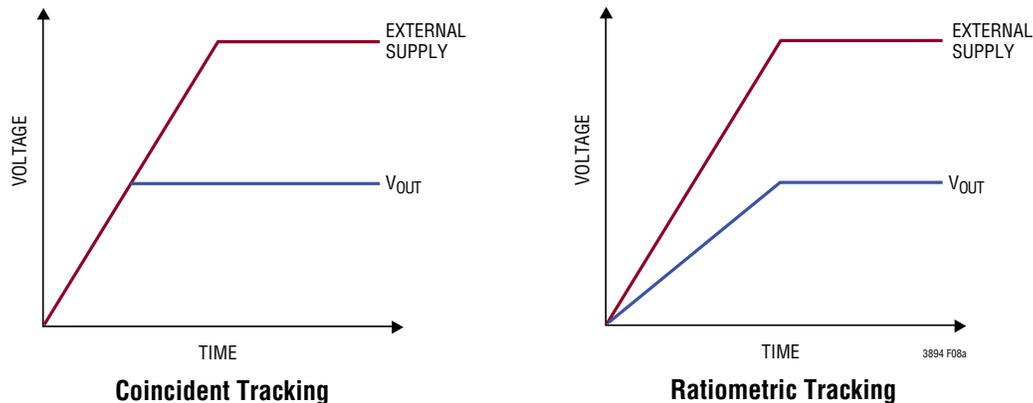
Figure 8(a). Two Different Modes of Output Tracking
