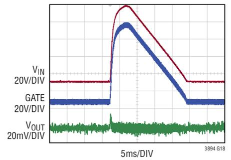
$V_{IN} = 12\text{V}$ , SURGE TO 100V
