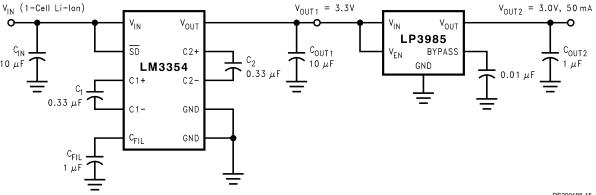
FIGURE 3. Low Output Noise and Ripple Buck/Boost Regulator
