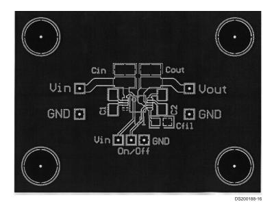
FIGURE 5. Typical Layout, Top View (magnification 1.5X)
