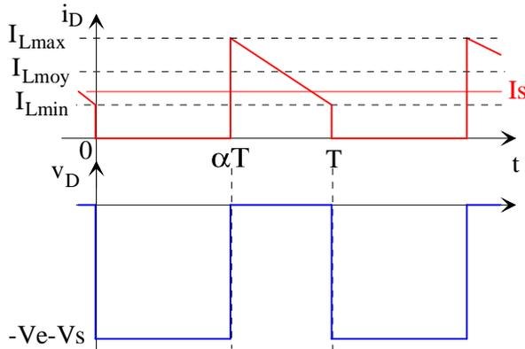
$$I_{D \max} = I_{FRM} = \langle i_L \rangle + \frac{\Delta I_L}{2}$$
