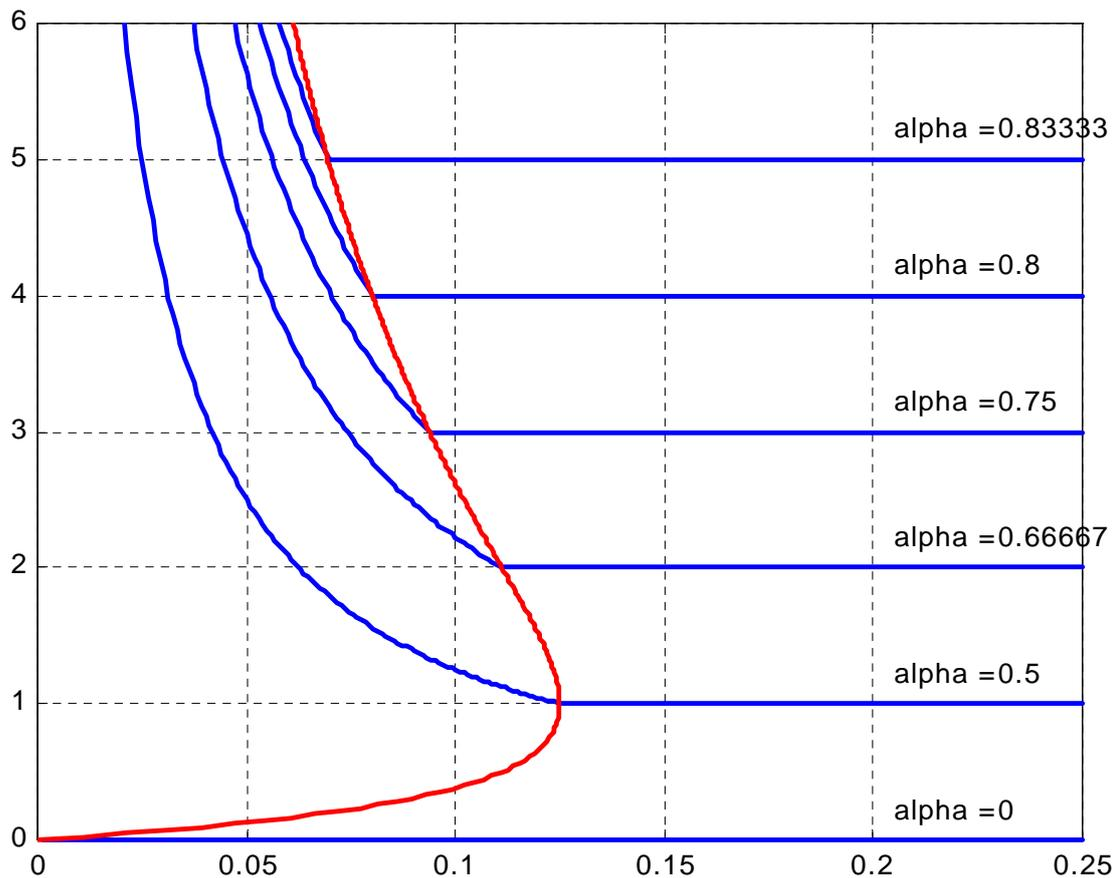
$$I_{s\text{limite}} = \frac{I_{L\text{max}}}{2} \alpha' = \frac{V_e}{2LF} \cdot \alpha(1-\alpha) ; x_{\text{limite}} = \frac{y}{2 \cdot (1+y)^2} ; \begin{cases} x_{\text{limite}} = \frac{\alpha \cdot (1-\alpha)}{2} \\ y_{\text{limite}} = \frac{\alpha}{1-\alpha} \end{cases}$$
