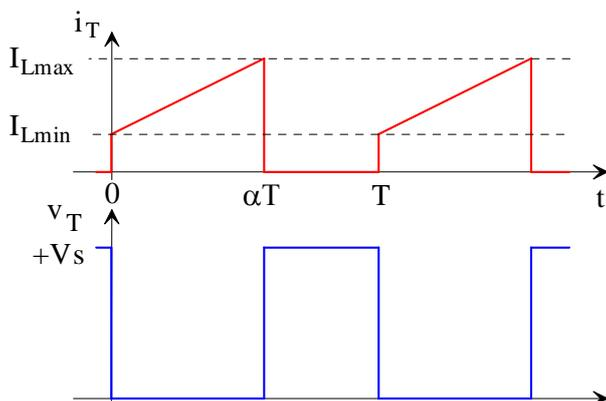
$$I_{T\max} = I_{D\max} = \frac{I_s}{1-\alpha} + \frac{\alpha \cdot V_e}{2LF}$$
