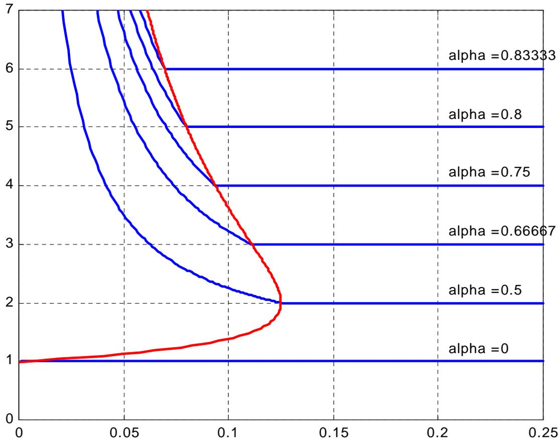
$$I_{s\text{limite}} = \frac{I_{L\text{max}}}{2} \alpha' = \frac{V_e}{2LF} \cdot \alpha(1-\alpha) ; x_{\text{limite}} = \frac{y-1}{2 \cdot y^2} ; \begin{cases} x_{\text{limite}} = \frac{\alpha(1-\alpha)}{2} \\ y_{\text{limite}} = \frac{1}{1-\alpha} \end{cases}$$
