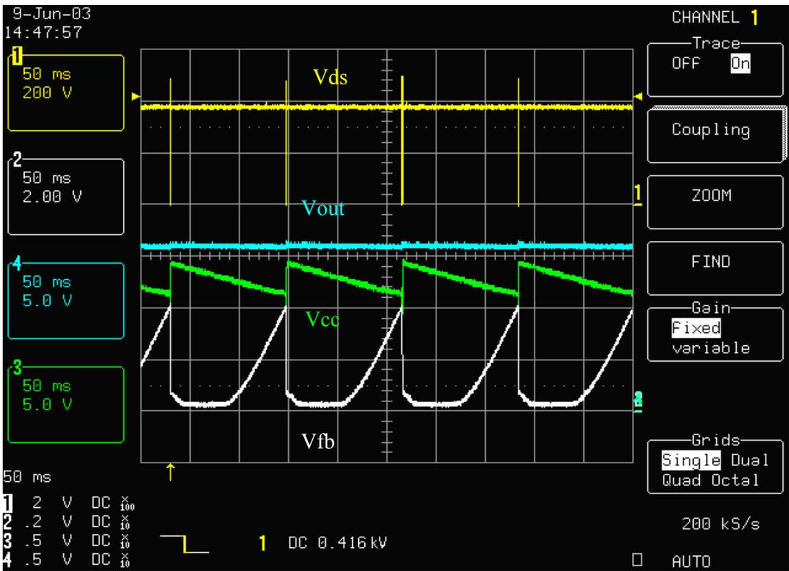
Burst Mode with No Load at Input Voltage 265V
