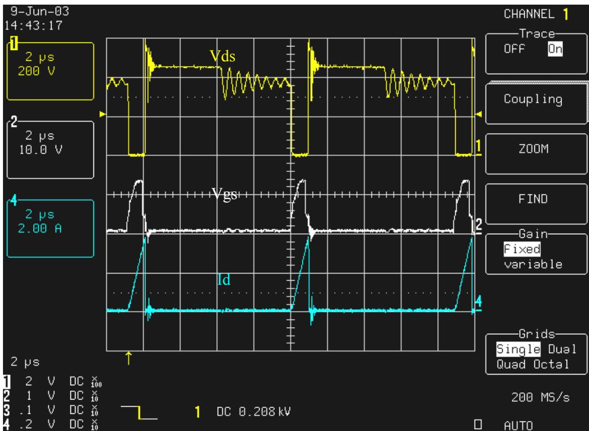
Normal Mode with Full Load 3.75A at Input Voltage 265V
