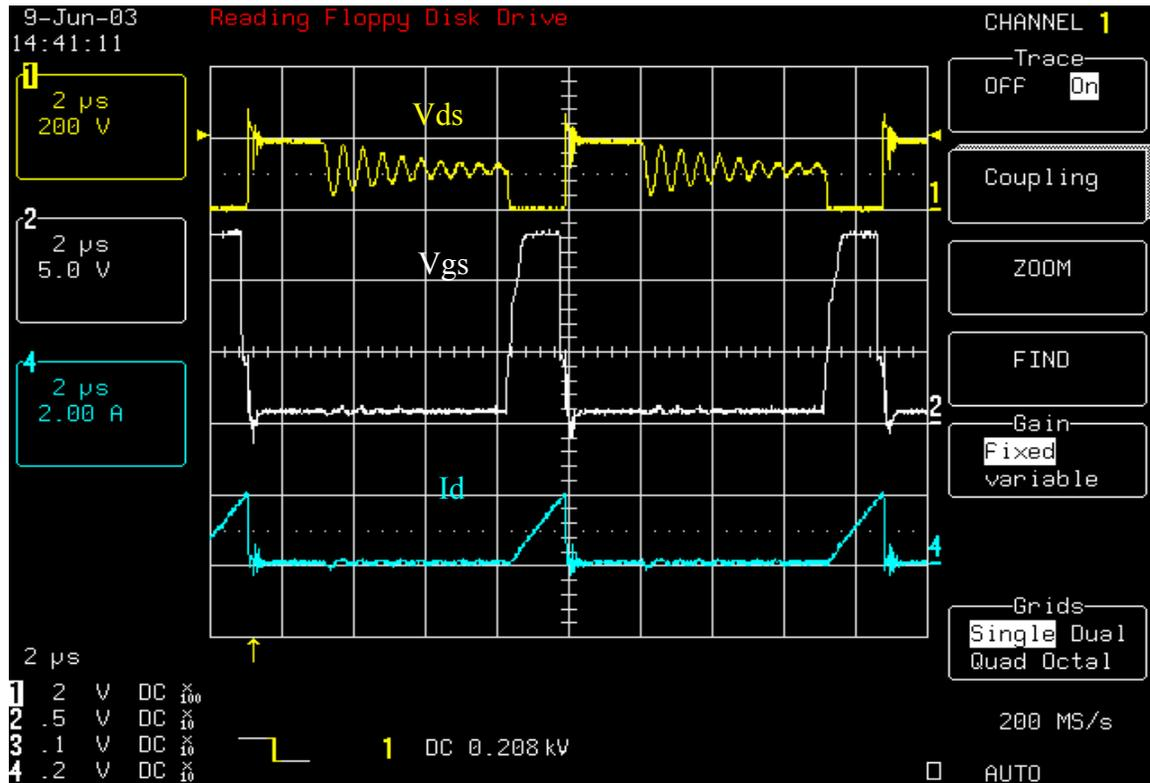
Normal Mode with 1A Load at Input Voltage 85V
