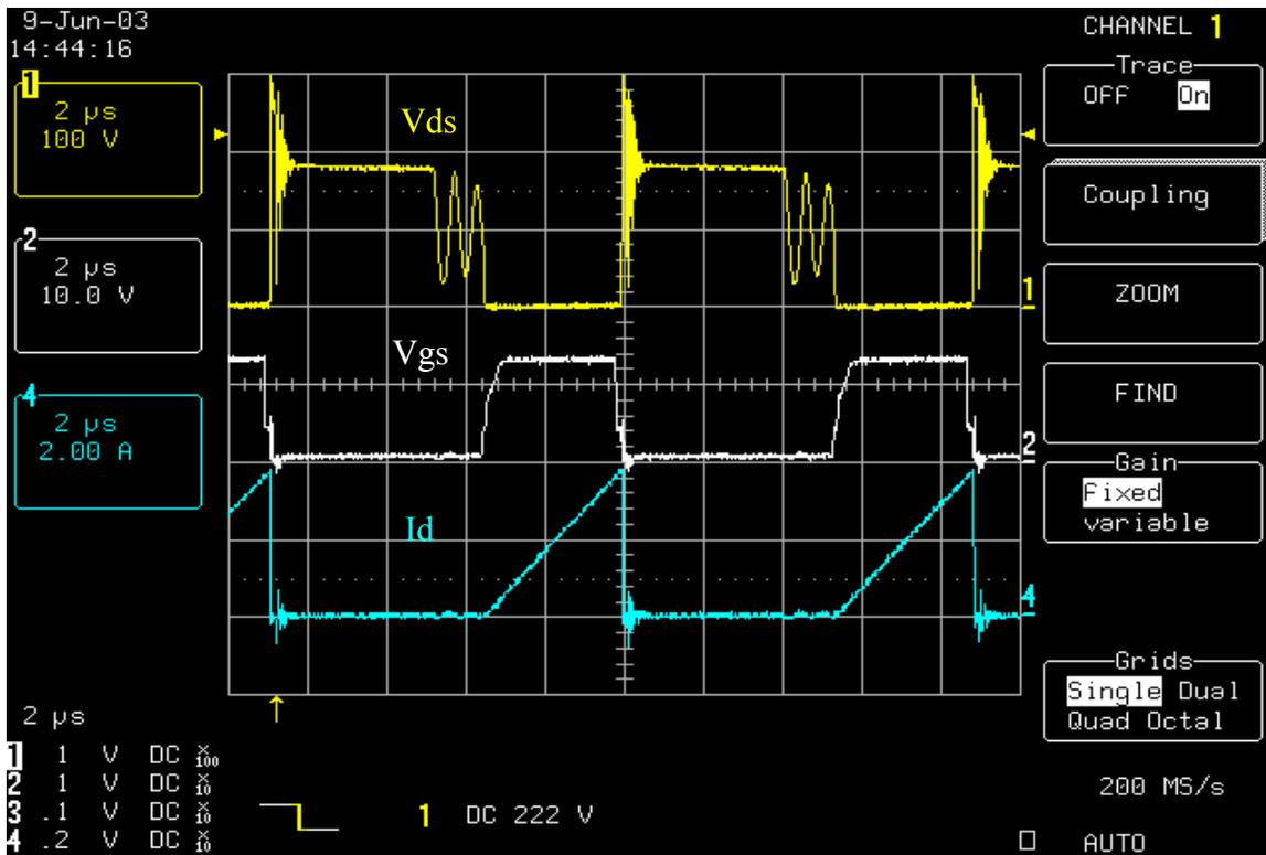
Normal Mode with Full Load 3.75A at Input Voltage 85V
