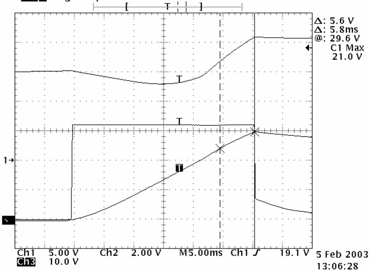
**Fig. 2: Overvoltage due to Open Loop**
