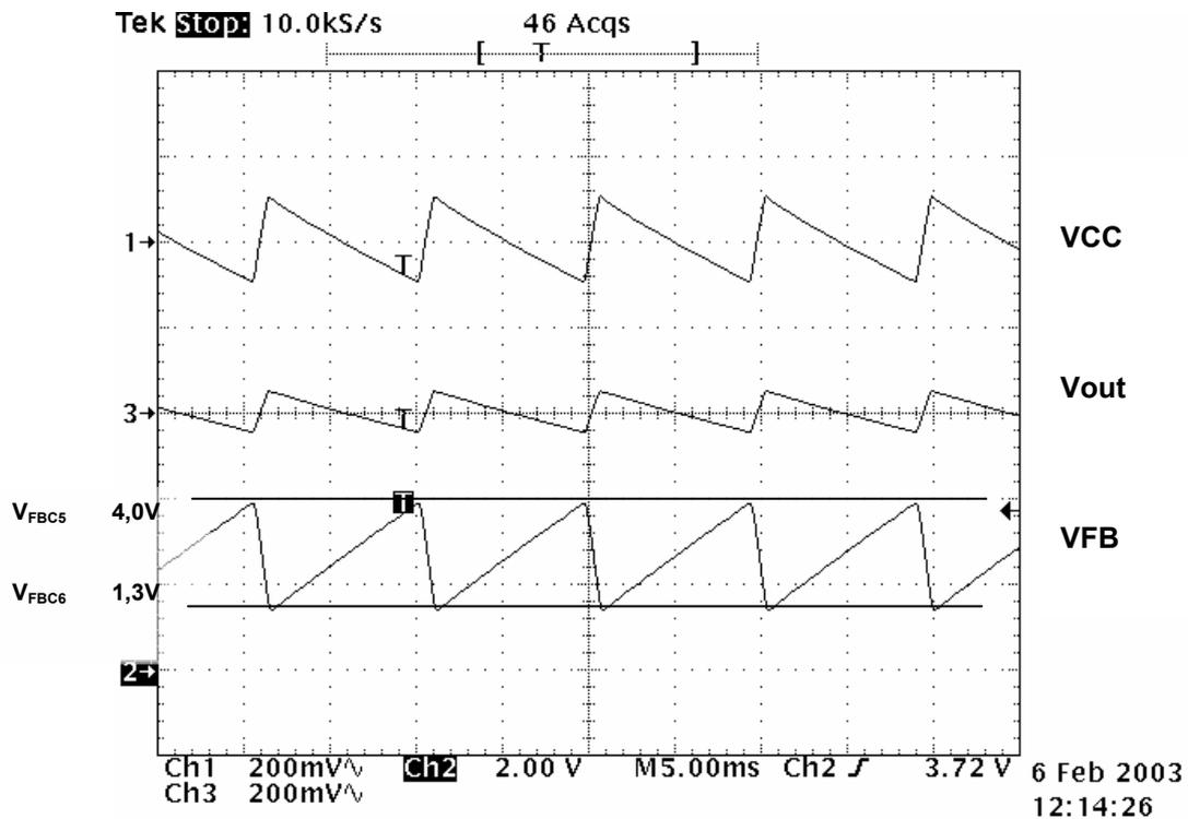
**Fig. 2: Burst Mode operation at 85Vac with lowload condition**
