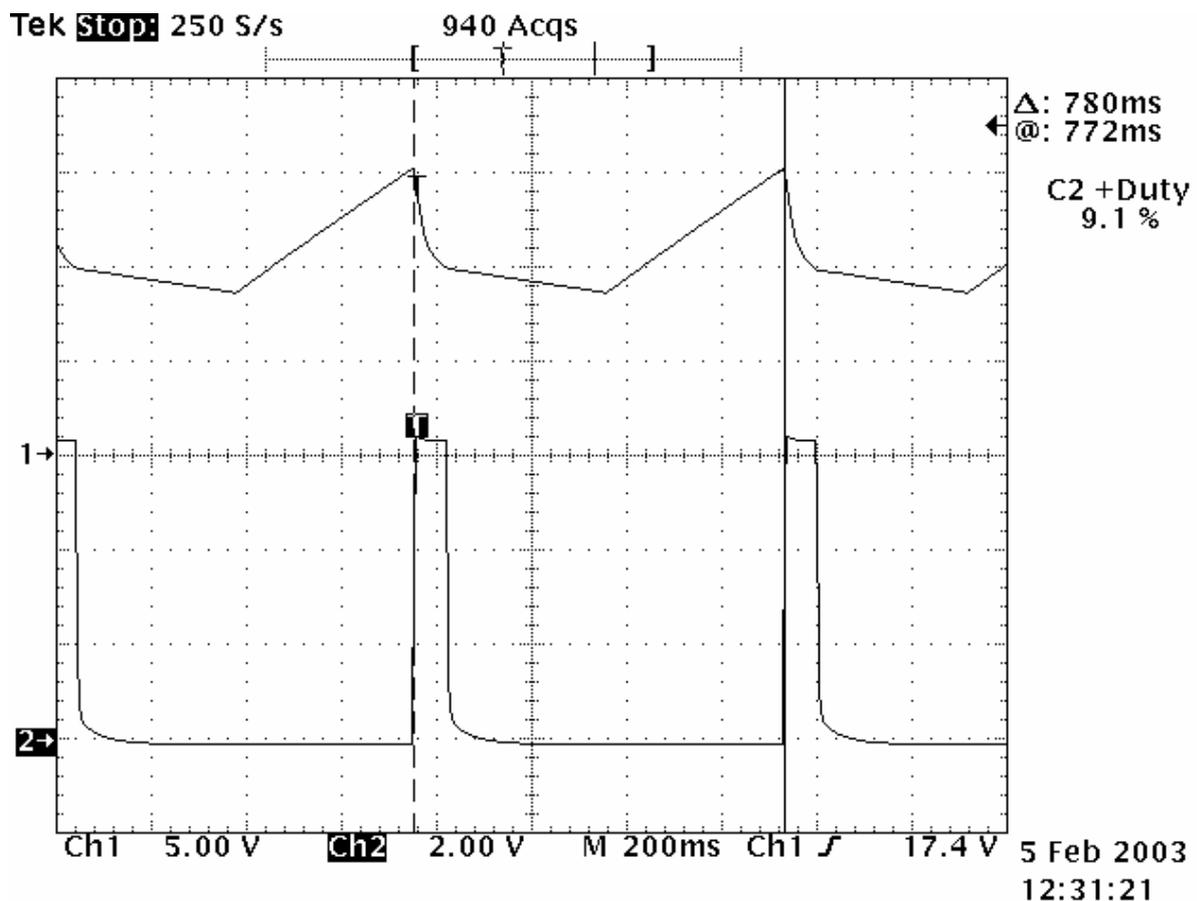
**Fig. 1: Short Circuit @ Output**
