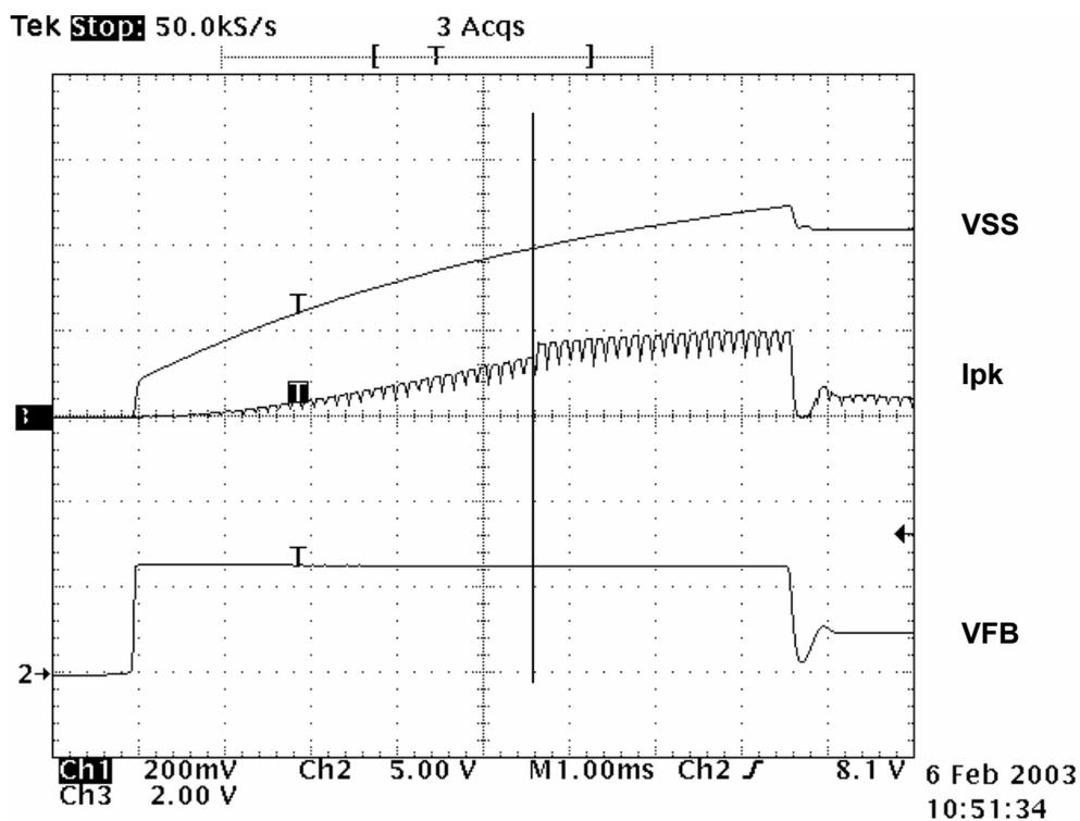
**Fig. 3: Softstart behaviour with nominal load**
