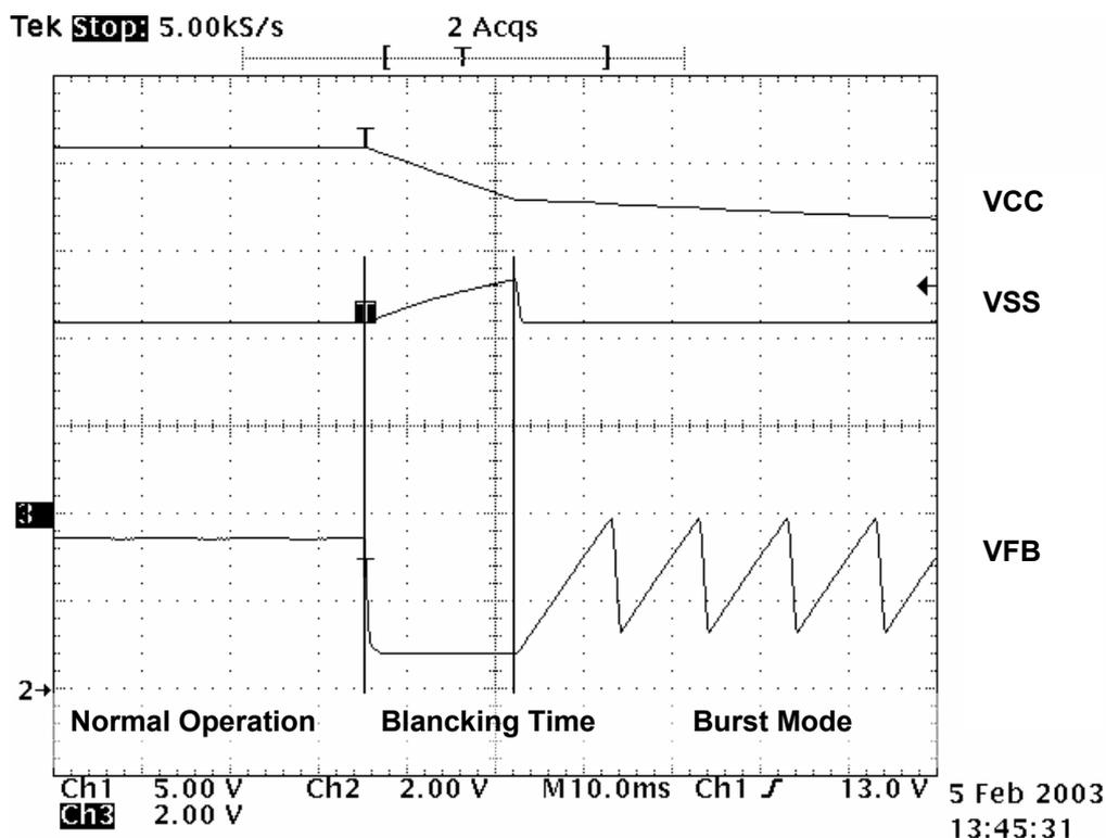
**Fig. 1: Jump from normal operation to Burst Mode**
