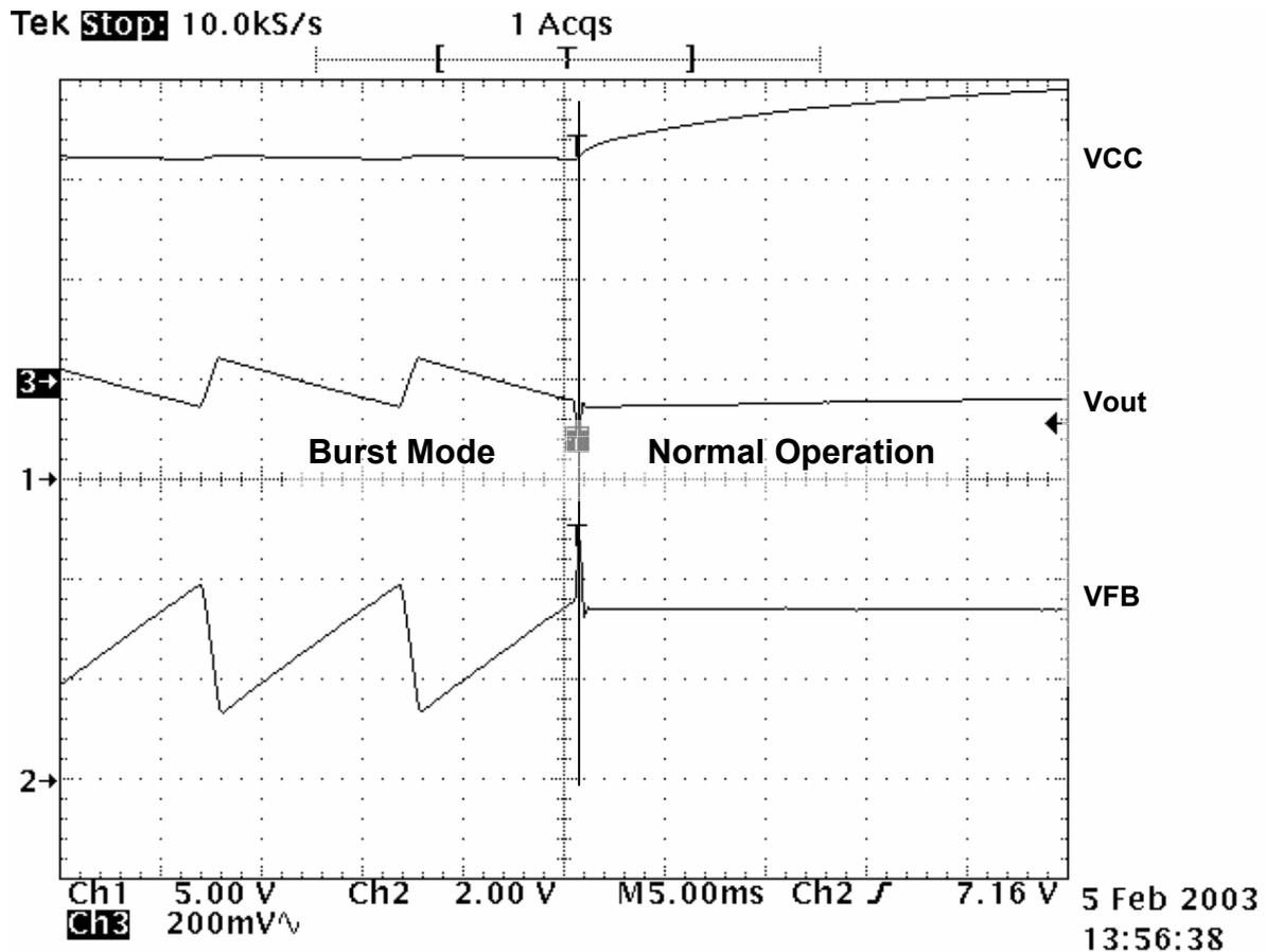
**Fig. 3: Load Jump from low load to nominal load.**
