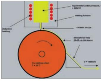
*Figure 1: Principle of rapid quenching technology*
