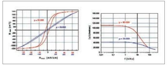
Figure 2: Variable range of hysteresis loops and permeability levels
