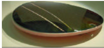
Warpage caused by wafer thinning: 200mm wafer thinned to 50 \mu\text{m}
