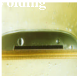
Chip on Board Globtop Voiding
