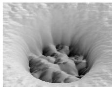
0.3μm W plug after CMP showing recess.
