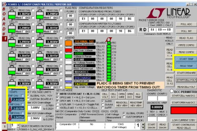
The LTC6803-1 has three ADC channels dedicated to measuring temperature. The temperature indications are for the internal die temperature of the LTC6803-1 and two externally connected thermistors. The display returns a voltage measurement.
