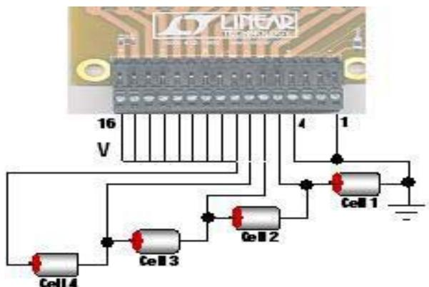
Figure 1. Connection of four cells (cell voltages at least 2.5V)
