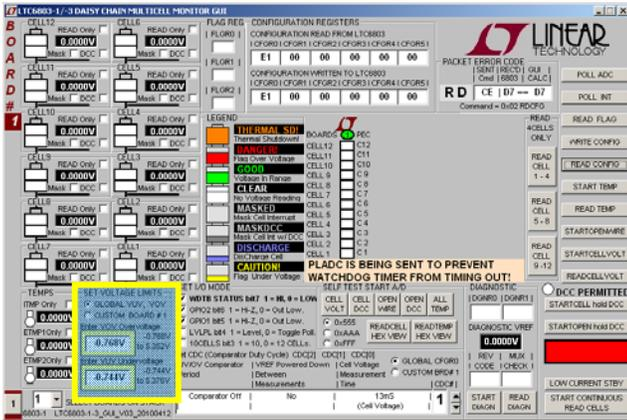
In the section labeled **SET VOLTAGE LIMITS** click on the boxes and enter voltage values for the over-voltage and under-voltage thresholds required for the cells being monitored. The voltage value entered will be rounded to the actual value used by the LTC6803-1 and displayed in the box. The voltage ranges for these thresholds is -0.74V to 5.35V and the program will not allow the under to be greater than the over voltage threshold.
