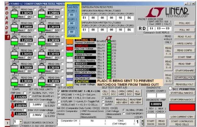
If the measured voltage of a cell is within the monitoring thresholds all indications for the cell appear green.
