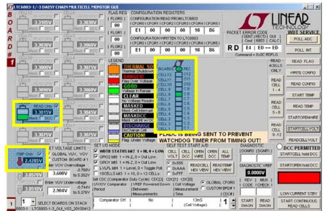
Each cell and each temperature channel has a check box to allow individual measurements. Checking these “Only” boxes sends the command (**STARTCELL VOLT** then **READCELL VOLT**, **START TEMP** then **READ TEMP**) to read only that channel and display its status. Cell 8 and Internal Temp are shown in the example screen above. Older or stale readings for all other cells and temperatures are faded out.
