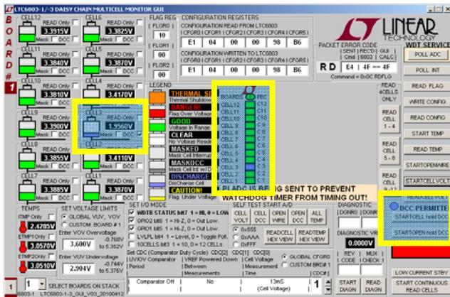
A check box is provided for each cell to be discharged. Checking this box (Cell 3 in the above example screen shot) and then writing the new configuration with a **WRITE CONFIG** button push will load the cell.
