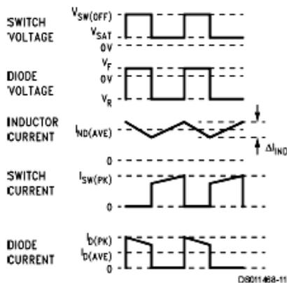
FIGURE 5. Step-Up Regulator Waveforms
