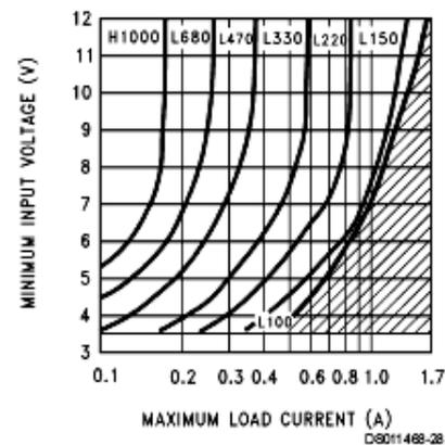
FIGURE 8. LM2577-15 Inductor Selection Guide
