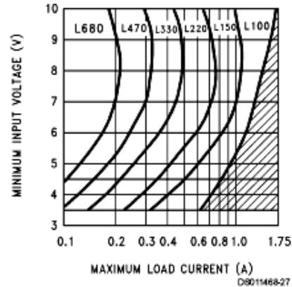
FIGURE 7. LM2577-12 Inductor Selection Guide
