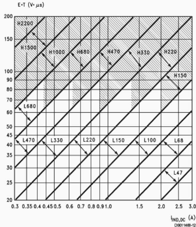
Note: These charts assume that the inductor ripple current is approximately 20% to 30% of the average inductor current (when the regulator is under full load). Greater ripple current causes higher peak switch currents and greater output ripple voltage; lower ripple current is achieved with larger-value inductors. The factor of 20 to 30% is chosen as a convenient balance between the two extremes.
