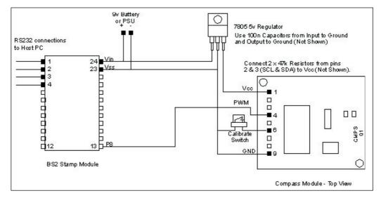
Note the switch connecting pin 6 to Ground. This is all that is needed for calibration of Rev7 Firmware.
