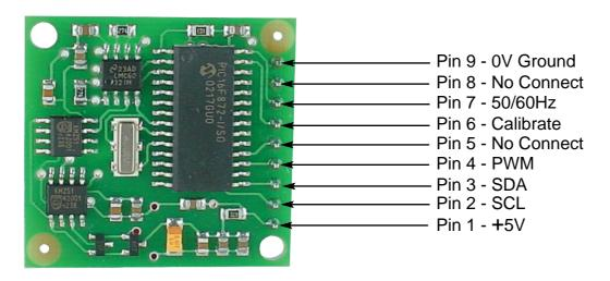
The compass module requires a 5v power supply at a nominal 15mA.
