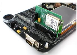
As explained in earlier section, USBizi (FEZ) can be used with modules with built in TCP/IP stack and socket support like the SparkFun shield with WiFly modules from Roving Networks.
