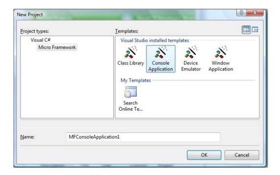
Click the "OK" button and you will have a new project that is ready to run. The project has only one C# file, called Program.cs, which contains very few lines of code. The file is shown in "Solution Explorer" window. If this window is not showing then you can open it by clicking "View->Solution Explorer" from the menu.
