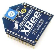
The modules have a very simple interface that runs on UART. With UART, the modules can be interfaced to any NETMF device. If creating a connection between two modules then XBee modules establish a connection automatically. If connecting multiple nodes then we would need to send some serial commands to configure our network. I suggest you start with automatic point-to-point connection.
