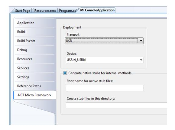
Pressing F5 will now send our simple application to FEZ and it will run right inside the real hardware. Switching from emulator to real hardware is that simple!
