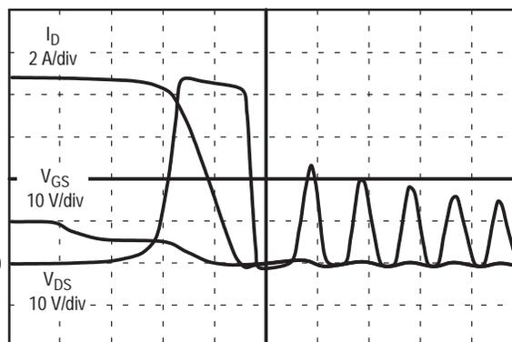
Figure 8b. Simulated Turn Off of an MTP15N06V at 116°C (250 ns/div)
