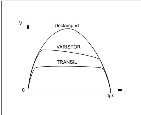
**Figure 2. Camp voltage versus overload current**
