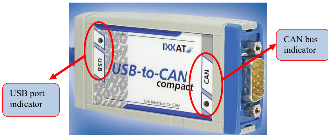
Fig. 64. The compact USB-to-CAN interface IXXAT [6].
