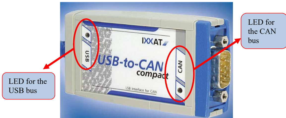
Fig. 1. The IXXAT USB-to-CAN interface [6].
