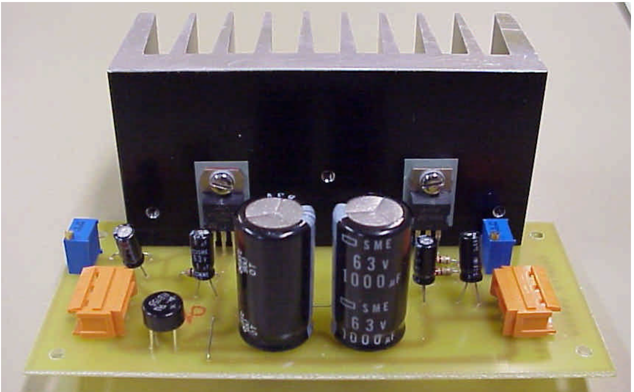
Figure 12.1. Alimentations +16V / -16V variables (images_maquettes\alim2-11.jpg).
