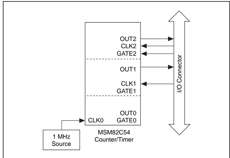
**Figure 4-2.** 516 Devices and DAQCard-500 Counter/Timer Signal Connections
