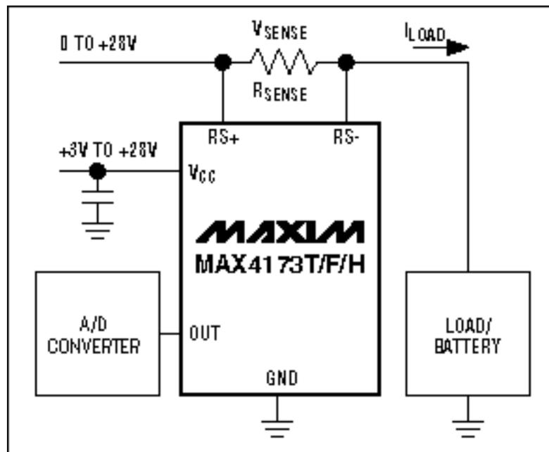
Figure 2. Example of a high-side current monitor
