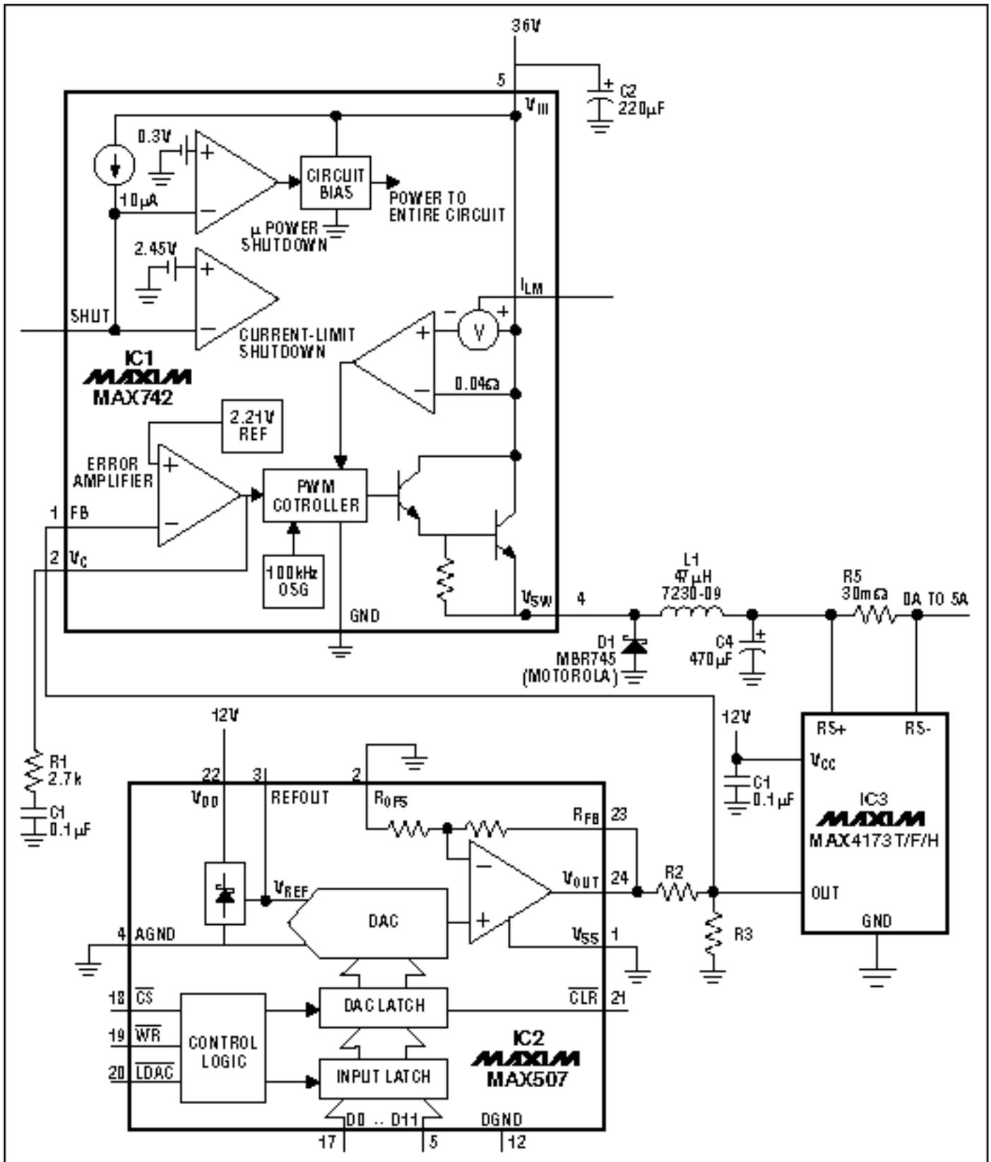
Figure 12. A 0-5A programmable current source (MAX4173)
