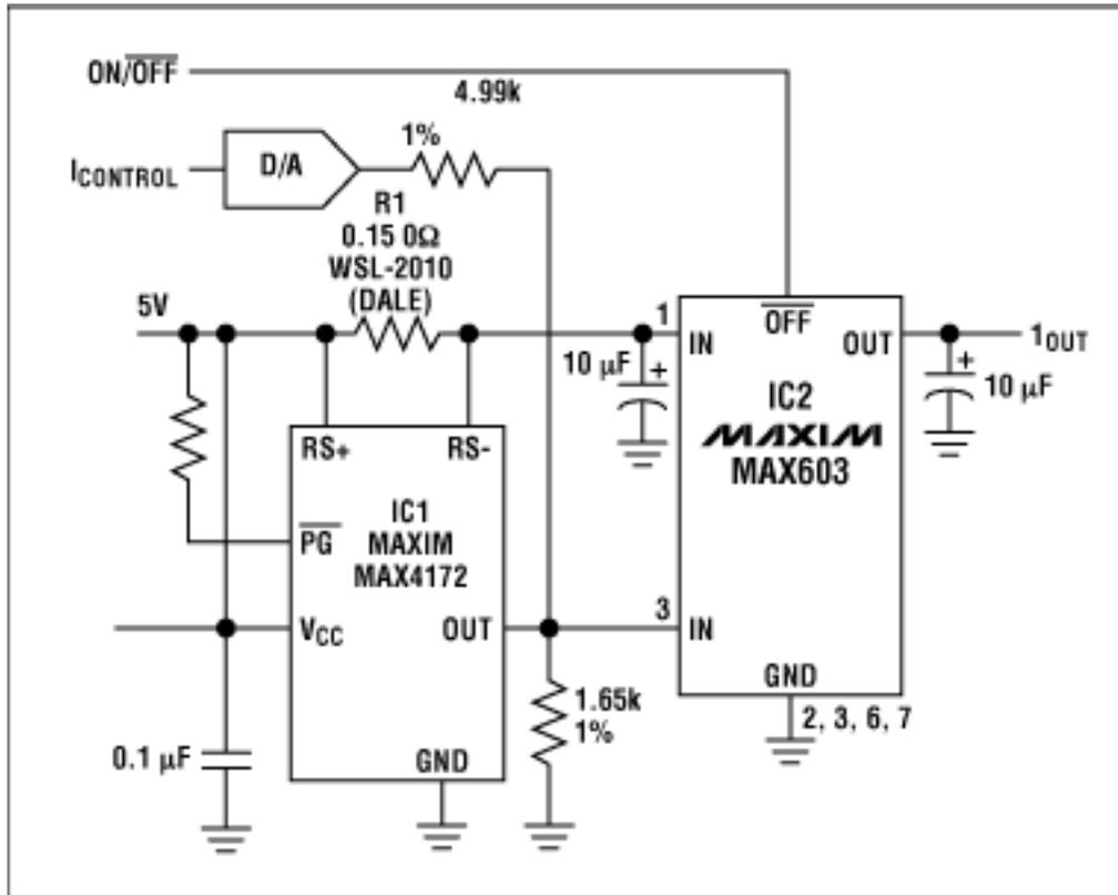
Figure 11. A variable, linear current source (MAX4173)
