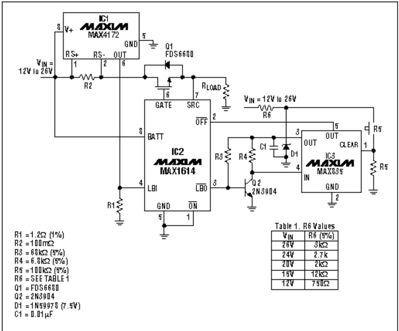
Figure 13. This high-voltage circuit breaker (MAX4172) protects to 26V.
