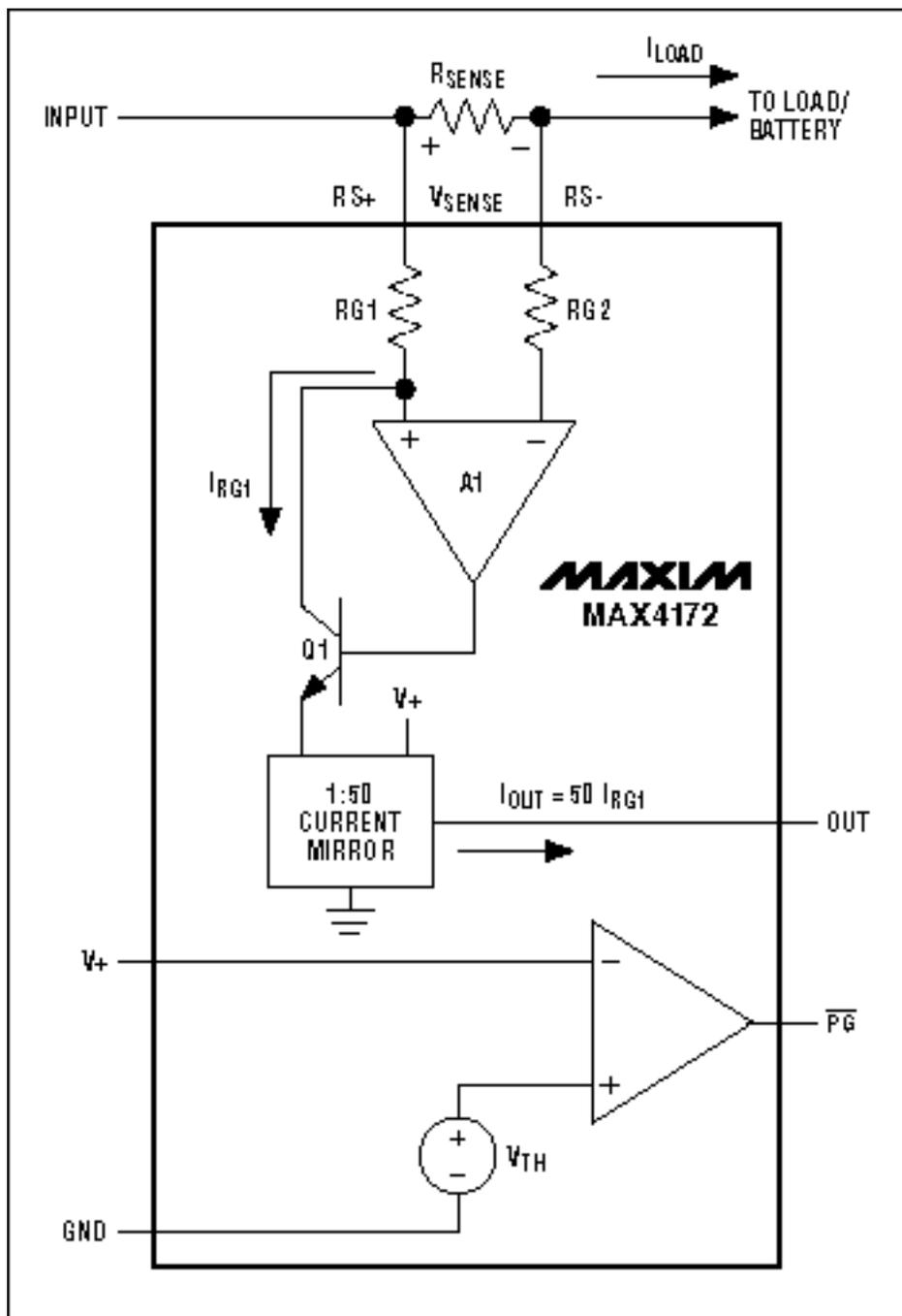
Figure 8. Another unidirectional high-side current monitor (MAX4172)
