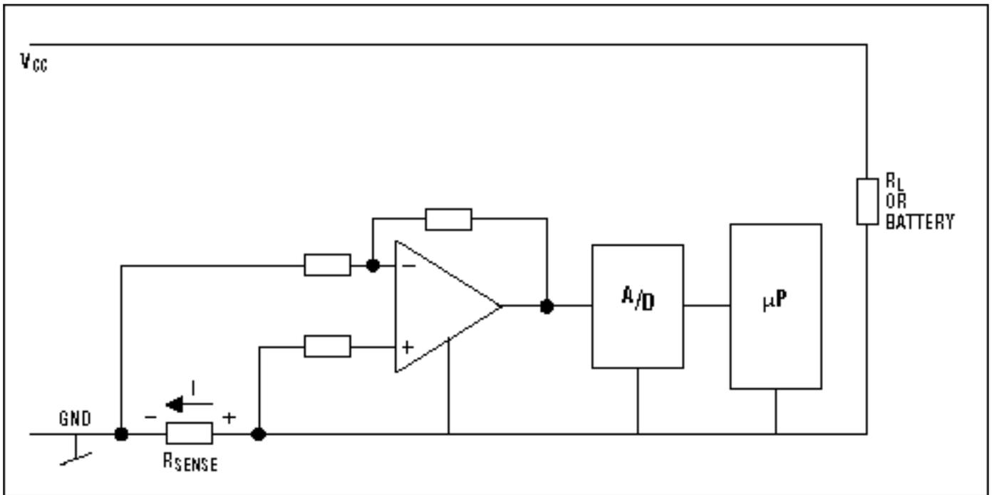
Figure 1. Principle of the low-side current monitor
