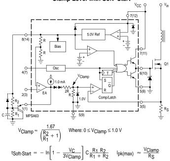
Figure 22. Current Sensing Power MOSFET
