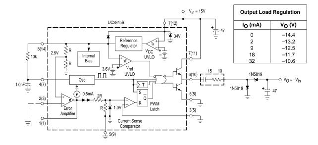
Figure 31. Voltage–Inverting Charge Pump Converter
