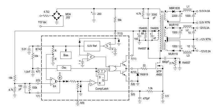
T1 – Primary: 45 Turns #26 AWG Secondary ±12 V: 9 Turns #30 AWG (2 Strands) Bifiliar Wound Secondary 5.0 V: 4 Turns (six strands) #26 Hexfiliar Wound Secondary Feedback: 10 Turns #30 AWG (2 strands) Bifiliar Wound Core: Ferroxcube EC35–3C8 Bobbin: Ferroxcube EC35PCB1 Gap: ≈ 0.10" for a primary inductance of 1.0 mH L1 – 15 μH at 5.0 A, Coilcraft Z7156
