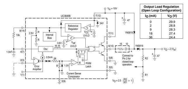
The capacitor's equivalent series resistance must limit the Drive Output current to 1.0 A. An additional series resistor may be required when using tantalum or other low ESR capacitors. The converter's output can provide excellent line and load regulation by connecting the R2/R1 resistor divider as shown.
