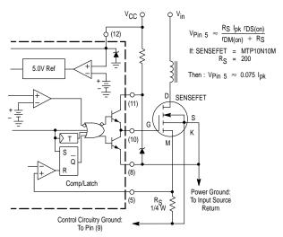
Virtually lossless current sensing can be achieved with the implementation of a SENSEFET power switch. For proper operation during over–current conditions, a reduction of the  $l_{pk}(max)$  clamp level must be implemented. Refer to Figures 19 and 21.
