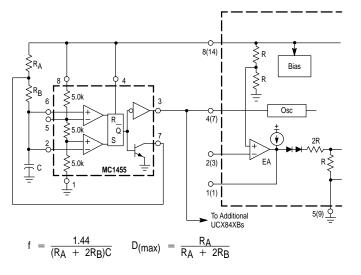
Figure 19. Adjustable Reduction of Clamp Level
