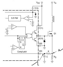
The addition of the RC filter will eliminate instability caused by the leading edge spike on the current waveform.
