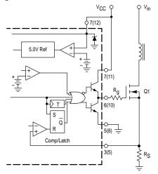
Series gate resistor  ${\sf R}_g$  will damp any high frequency parasitic oscillations caused by the MOSFET input capacitance and any series wiring inductance in the gate–source circuit.
