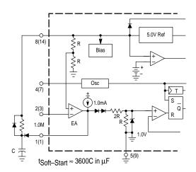
Figure 21. Adjustable Buffered Reduction of Clamp Level with Soft–Start
