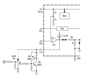
The MCR101 SCR must be selected for a holding of < 0.5 mA @ T\_A(min). The simple two transistor circuit can be used in place of the SCR as shown. All resistors are 10 k.
