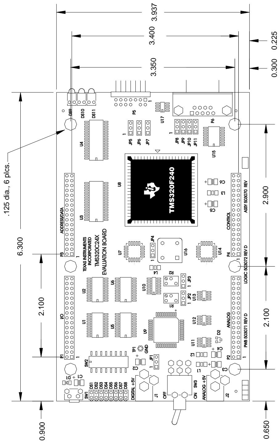
Figure A-2. Schematic Diagram of the TMS320C24x Evaluation Board
