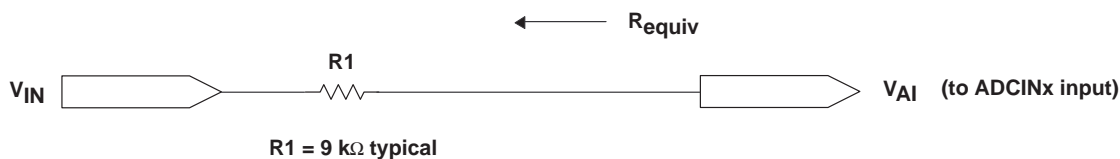
Figure 47. Typical ADC Input Pin Circuit
