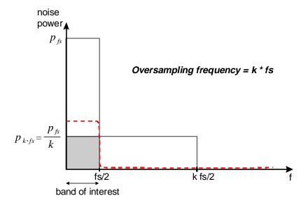
Digital low-pass filters should remove all frequencies above  $f_s/2$ . The effective resolution is determined by the quality of the digital filter. The remaining noise power beyond  $f_s/2$  is a measure for the quantization noise and therefore responsible for a decrease in the signal-to-noise ratio (SNR).
