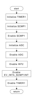
In order to generate interrupts constantly from timer 1, CPU interrupt INT2 and the peripheral level interrupt from timer 1 (EV\_INTA\_T1PINT) are enabled. An interrupt service routine responding on INT2 interrupts will be installed to drive further steps of the signal generation, data acquisition and calculations.
