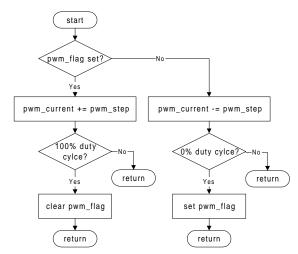
The PWM duty cycle should range between 0 and 100% in order to achieve the highest possible resolution. The duty cycle is programmed by setting up the simple compare register (SCMPR1).
