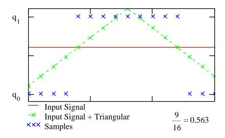
In general the following equation applies to a triangular modulated oversampling:
