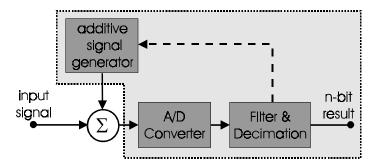
The devices of the TMS320C24x family includes all components drawn in the dotted block, which simplifies the design of such an oversampling subsystem.
