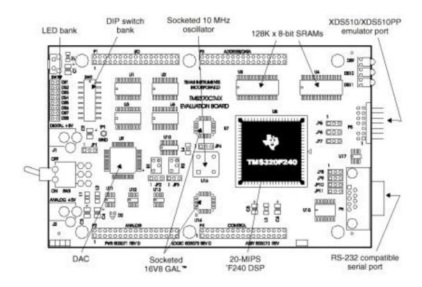
The evaluation board can be controlled and debugged through the board's JTAG Interface using any Texas Instruments XDS510 emulator.
