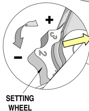
1. Hold the hand tool in the palm of your hand as shown in Figure 10. Using the index finger squeeze the link towards the top of the hand tool frame. This will release the preload adjustment wheel.
