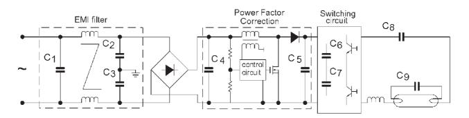
The increasing switching frequency of electronic ballasts in the range of 60 to 150 KHz takes advantage in performances applaying Polypropylene film capacitors C 5 in replacement of electrolytics capacitors.
