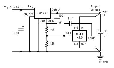
FIGURE 7. Precision 5V 1A Low Dropout Regulator
