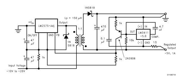
FIGURE 6. Negative Input, Negative or Positive Output Flyback Regulator
