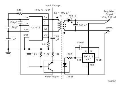
FIGURE 3. Isolated 250 mA Flyback Switching Regulator
