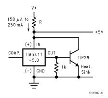
FIGURE 14. 250 mA Shunt Regulator
