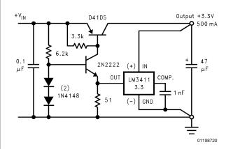
FIGURE 8. 3.3V 0.5A Low Dropout Regulator
