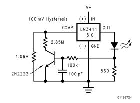
FIGURE 12. 4.7V Power ON Detector with Hysteresis
