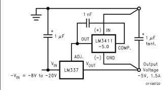
FIGURE 10. Precision Negative Voltage Regulator
