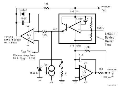
FIGURE 2. LM3411 Test Circuit
