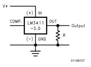
FIGURE 15. Voltage Detector
