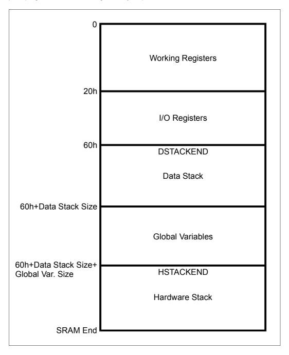
The **Working Registers** area contains 32x8 bit general purpose working registers. The compiler uses the following registers: R0, R1, R15, R22, R23, R24, R25, R26, R27, R28, R29, R30 and R31.
