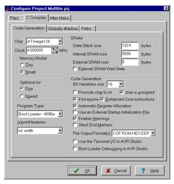
If this option is enabled, the compiler will generate supplementary code that allows the Boot Loader to be source level debugged in the AVR Studio simulator/emulator.
