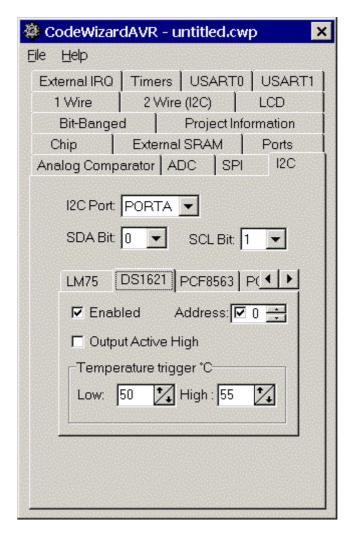
The **Output Active High** check box specifies the active state of the DS1621 Tout output. The **Low**, respectively **High**, spinedit boxes specify the low, respectively high temperatures trigger temperatures for the Tout output.
