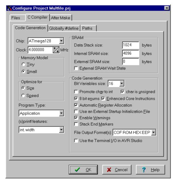
You can select the target AVR microcontroller chip by using the **Chip** combo box. You must also specify the **CPU Clock Frequency** in MHz, which is needed by the Delay Functions, 1 Wire Protocol Functions and Dallas Semiconductor DS1820/DS18S20 Temperature Sensors Functions.
