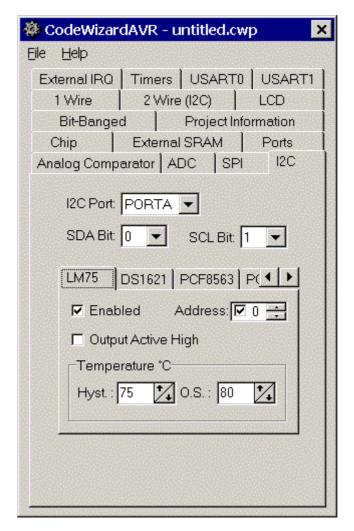
The **LM75 Address** list box allows you to specify the 3 lower bits of the I<sup>2</sup>C addresses of the LM75 devices connected to the bus. Maximum 8 LM75 devices can be used.
