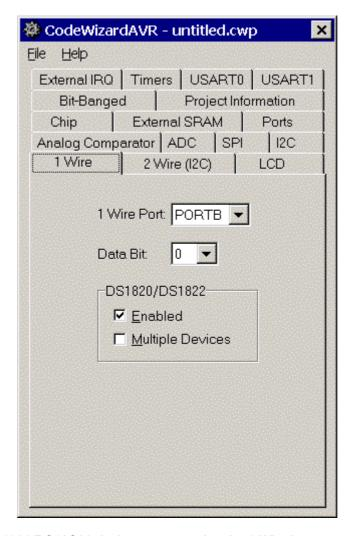
If you use several DS1820/DS18S20 devices connected to the 1 Wire bus, you must check the **Multiple Devices** check box. Maximum 8 DS1820/DS18S20 devices can be connected to the bus. The ROM codes for these devices will be stored in the **ds1820\_rom\_codes** array.
