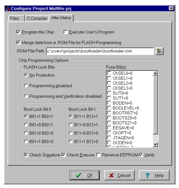
If you check the **Program the Chip** option, then after successful compilation/assembly your program will be automatically transferred to the AVR chip using the built-in Programmer software.
