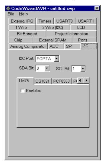
Using the  $I^2C$  Port list box you can specify which port is used for the implementation of the  $I^2C$  bus. The SDA Bit and SCL Bit list boxes allow you to specify which port bits the  $I^2C$  bus uses.
