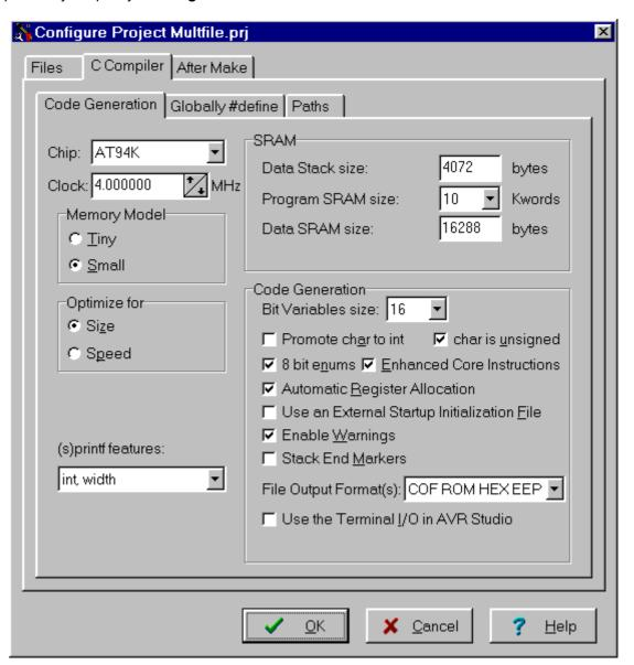
The size of the bit variables, which are placed in registers R2 to R14, can be specified using the **Bit Variables size** list box.
