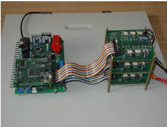
1kVA Matrix Converter
