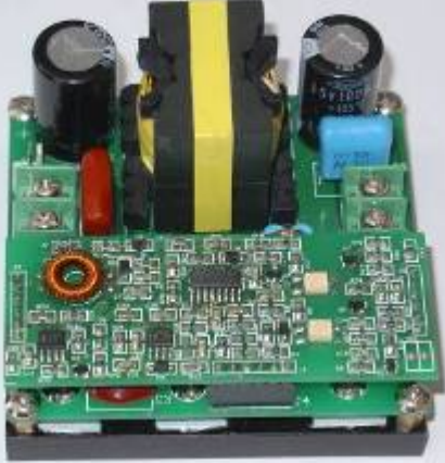
100VA DC/DC Converter
