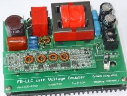
500VA DC/DC Converter
