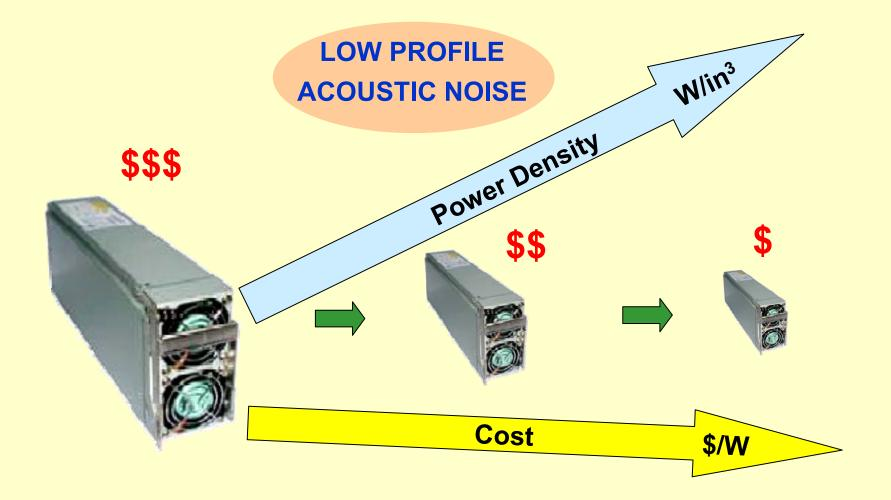
• Power-supply technology will continue to be primarily driven by extremely challenging power-density requirements that need to be met in cost-effective way
