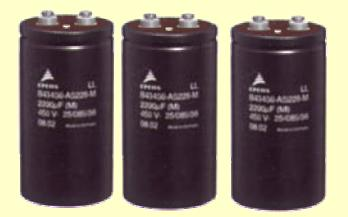
two caps required to meet hold-up time requirement however, three caps are required to handle ripple current to meet life time specs
