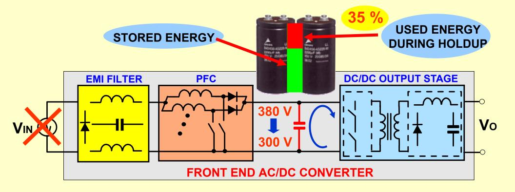
• Only approximately one-third of energy stored in bulk capacitor(s) is utilized during hold-up time
