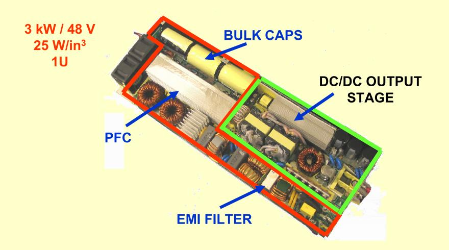
• Decreasing size of front end is key to increasing power density of ac/dc power supplies
