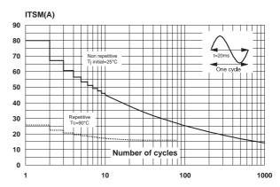
**Fig. 6:** Non repetitive surge peak on-state current for a sinusoidal pulse with width tp < 10ms, and corresponding value of  $l^2t$ .
